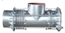
and a balanced bellows and elbow or tee, head, tie rod, end plate, spherical and tapered washer and other structures. It is mainly used to absorb the combined axial and lateral displacement and can balance the pressure and thrust of the bellows. Usually, the pipeline expansion joint is a constrained general-purpose type that can accept lateral movement. Because there is also axial deflection, pressure balanced elbows are usually required.
